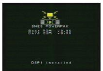
The intro screen also shows if you have the DSP1 chip installed. Hold the select button when you turn on your console to see a list of the versions of each chip inside.
