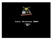
To save games stored in Battery RAM, hold the reset button on the console for 2-3 seconds to go back to the PowerPak menus. The PowerPak will not create new .sav files, only **overwrite** existing ones. You can get empty save files from the website.
