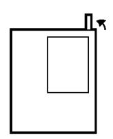
To remove the card, flip the ejector straight up.
